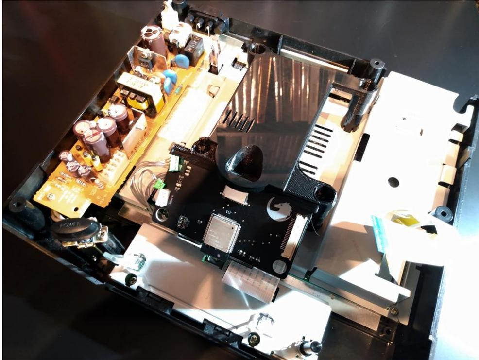
Once the mount is fully seated on the posts install the power and ribbon cable into the Fenrir:
