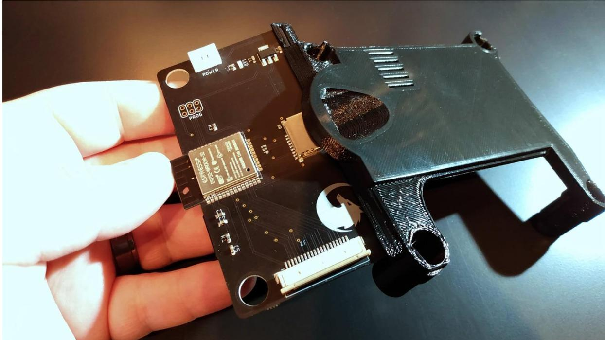
Once the top edge is in place, gently squeeze the Fenrir into hooks along the bottom of the mount and they should clip into place as shown:
