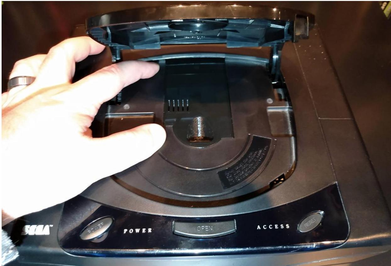
The top surface of the mount should be flush with the opening of the console case.
