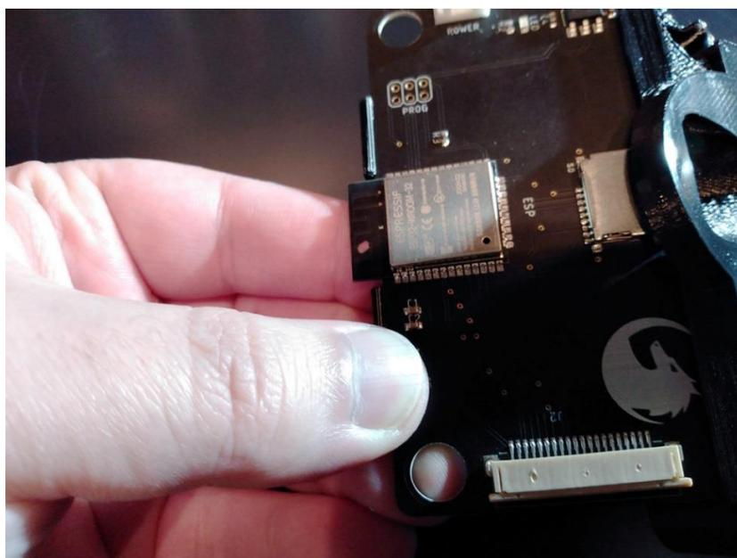
**Step 2: Install the Fenrir with Mount into the console.**
