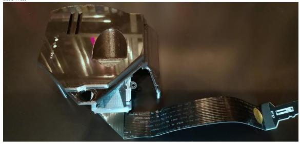
Ensure that the button extensions are installed into the bit-district SD Card Mount and place this assembly on top of the MODE PCB; then install the ribbon cable into the Micro SD Card Slot as shown.
