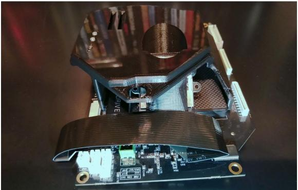
Ensure that the ribbon cable is folded as close to the Micro SD card adapter as possible as this will aide in clearance against the Dreamcast Power Supply.
