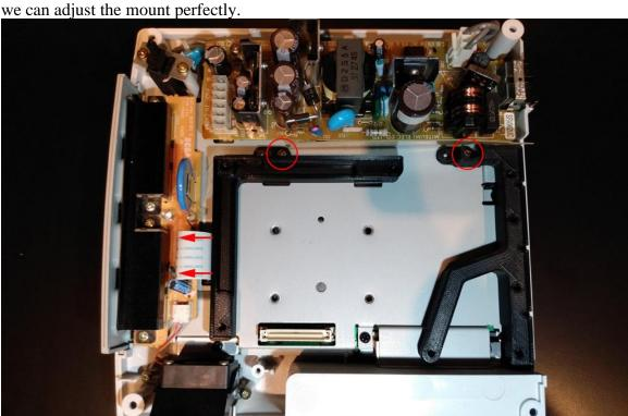
With the screws in the mount slightly lose and the ribbon cable pushed out of the way place the MODE into the mount and connector nudge the mount as necessary until the mode is fully seated into the mount and the connector.
