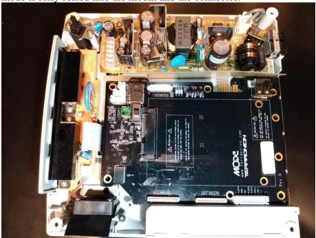
With the MODE Fully Seated tighten the screw by SD card slot, remove the mode, and then tighten the other screw.
