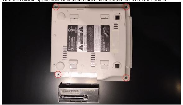
Once you have removed the 4 screws the upper shell should easily separate from the rest of the console. Put the screws and the upper shell aside for now.
