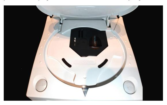
With everything aligned and in place you can close the Dreamcast's lid, turn it back upside down and re-install the 4 case screws and network adapter.
