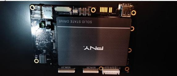
Once the drive is in place turn the MODE upside Down, Then you can install 2 of the 3mm screws that should have come with your SATA Drive to secure your drive to the MODE PCB.
