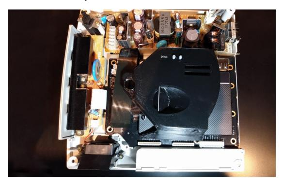
With the MODE fully seated into the connector and the PCB mount you can place the upper shell back on top of the Dreamcast console. You will want to open the lid so that you can more easily align the bit-district SD Card Mount with the opening in the shell.
