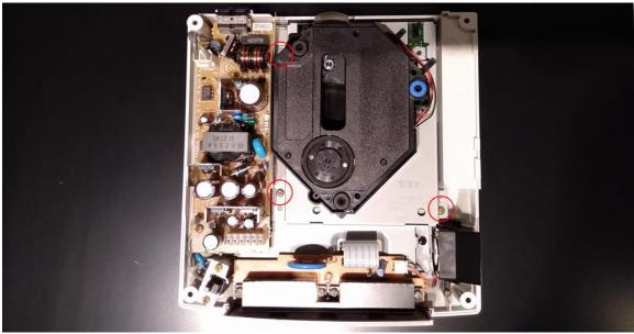
Once you have removed the 3 screws you should be able to pull the GD-ROM unit straight up to remove it from the Dreamcast. There is a connector near the corner by the cooling fan that will produce some resistance but it should remove with only gentile force.
