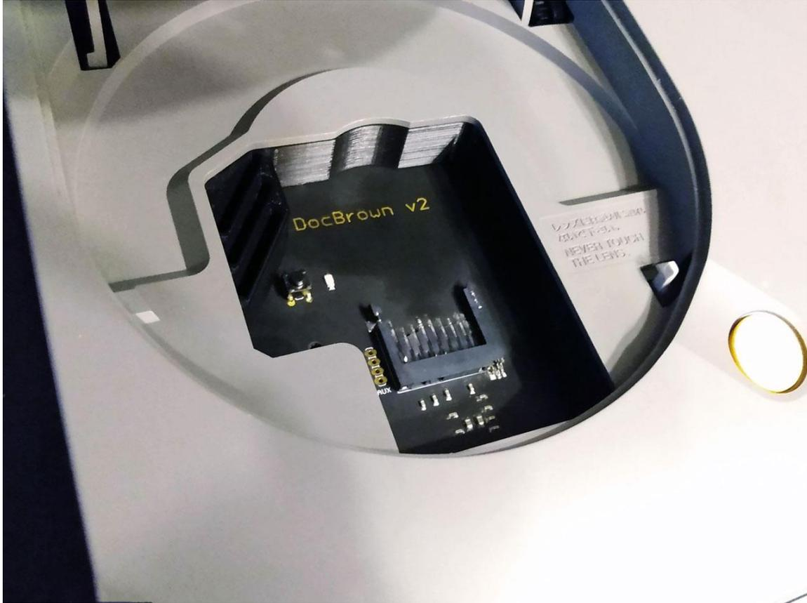
Once you're confident that everything is fully seated and aligned turn the console upside-down and re-install the 4-case screws.
