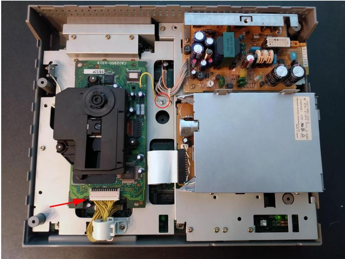
Once you have removed the screw and disconnect the connector you should be able to remove the CD-ROM drive straight up and off.
