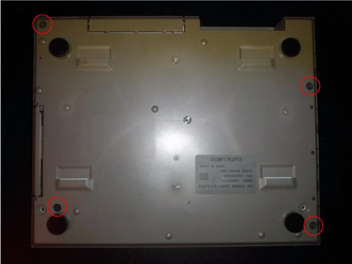
Once you have removed the 4 screws Push the Power button “ON”. The upper shell should easily separate from the rest of the console.
