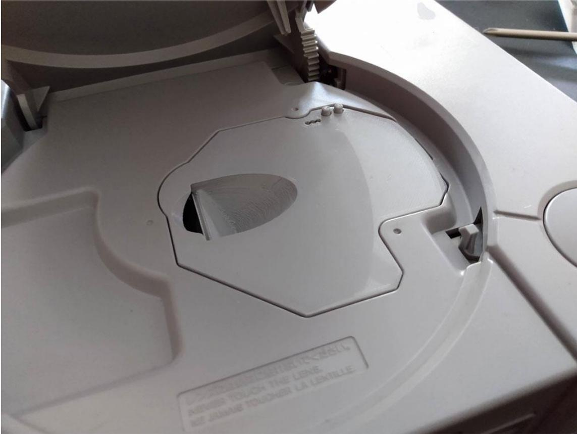
Once the Upper Console Case is fully seated you can turn it over and re-install the case screws as well as the Serial Port door.
